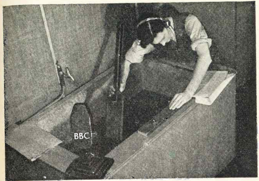
One way of producing sound effects: in this case the sound of a rowing boat. The water tank is in the studio, and the "jeep" operates a paddle while keeping a sharp eye on the script. Recorded effects are more usual, and are explained in the chapter on "Recorded Programmes."
