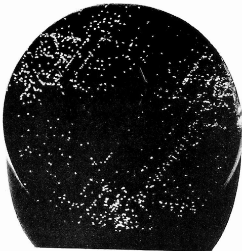
Fig. 5. Edge dislocation etch pits on a (111) silicon cross section. Mag. \times 4
