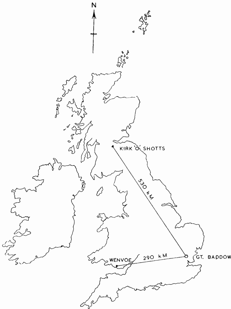
FIG. 1 Disposition of Transmitters with respect to receiving site.
