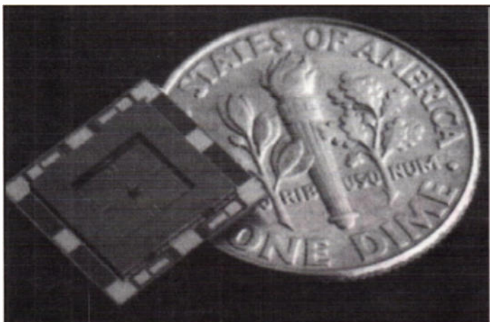
Figure 6 JPL Pasadena/Hughes miniaturised gyroscope for space stabilisation. Courtesy NASA.
