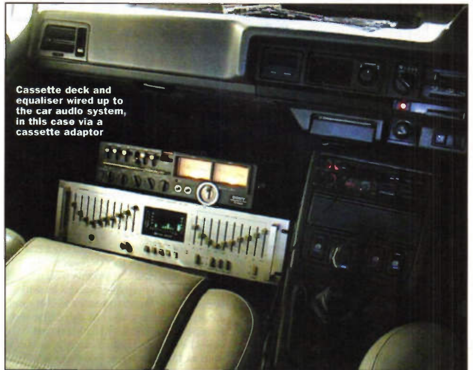
Figure 1. Wiring up the audio source and equaliser to the in-car sound system.
