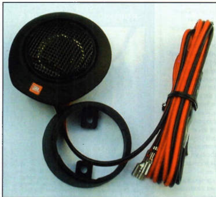
A pair of external tweeters, suitably located, can brighten up the sound considerably. This JBL model, which is sold by Maplin, benefits from flexible mounting options. Note the in-line capacitor, which 'blocks' lower frequencies.
