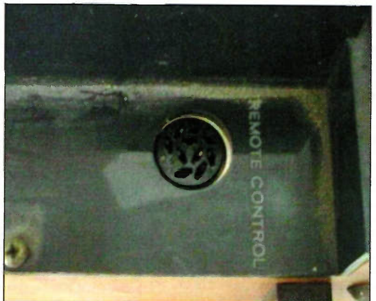
Photo 6. The A77 remote control socket. Pins 1 and 2 must be shorted in the absence of a remote control. Normally, this would be achieved by means of a 'blanking' plug.
