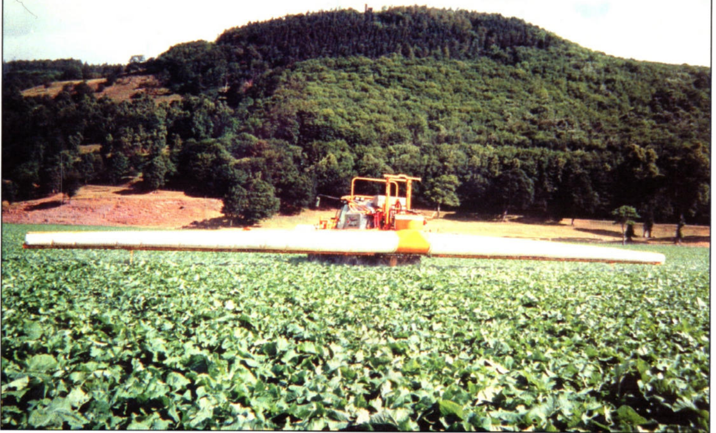
Photo 13. Knight wide boom air assisted sprayer (courtesy of Knight Farm Machinery Ltd.)
