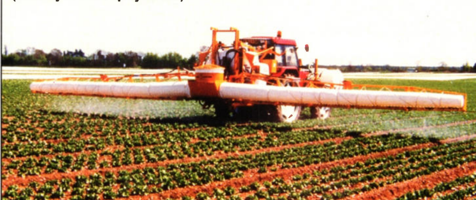
Photo 14. Hardi Air Assisted Sprayer. Note blower at centre of boom (courtesy of Hardi Sprayers Ltd.)
