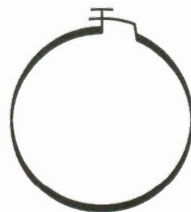
Figure 2. Hertz's receiving antenna - a Knochenhaur Coil.
