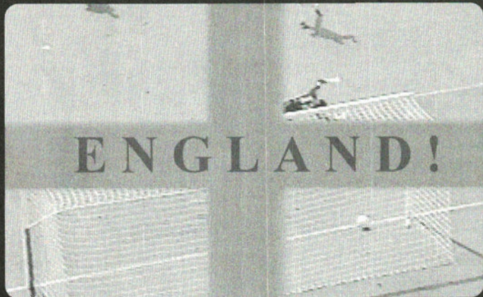
Red cross wipe, which moves out from centre to fill screen with red. Wipe is engaged by selecting all four horizontal and vertical wipe effects, together with 'Invert'. 'Angle' feature is turned off. The 'England!' caption was added using a title generator.
