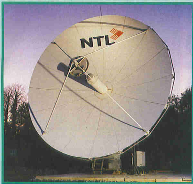
Photo 3. NTL's 8-metre uplink dish, used for experiments with MPEG transmission via satellite.
