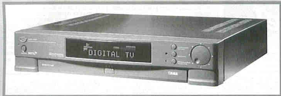
Photo 7. A prototype Pace/NTL receiver/decoder for MPEG-encoded satellite broadcasts from the proposed Digital Sky service.
