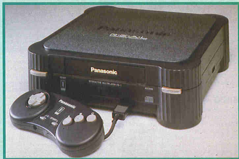
Photo 6. The 3DO multimedia games machine will shortly be able to play MPEG-encoded CD-Video discs by virtue of an MPEG cartridge (available from November).
