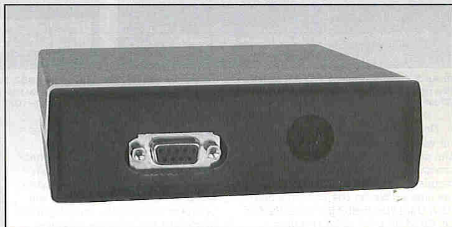
Rear panel of the Packet Radio MODEM showing the 9-way D-type and the 5-pin DIN connectors.
