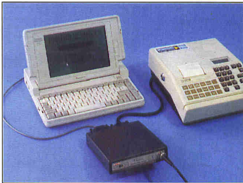
Top: Paknet in a retail application. Top Left: A Paknet Radio Pad. Note the compact size. Left: The Paknet Base Station, normally located at a cellular repeater site. Above: the Radio-Pad has two user ports, allowing for two completely independent applications. For example, one port may be connected to an EFTPoS terminal, the other possibly to a security system or computer.
