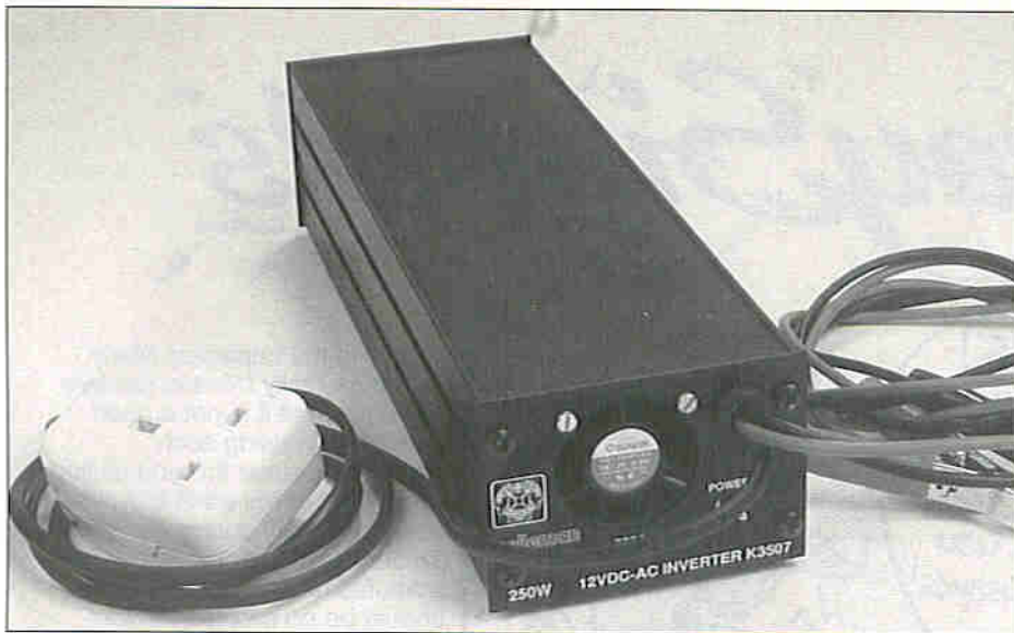
Photo 3. The completed 12V DC/230V AC Inverter, with wires attached.
