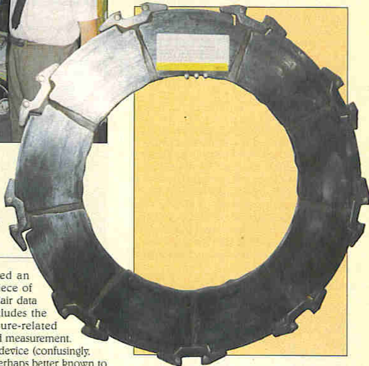
Above: Godfrey duly demonstrates the positioning system of the Ekco cloud radar dish. Right: A disc brake pad from a Boeing 737-200 passenger aircraft.
