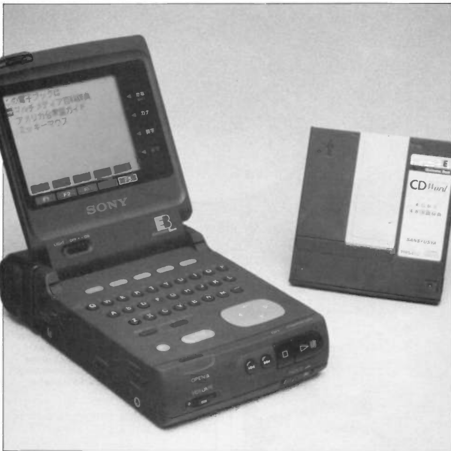
The Sony Data Discman, referred to as an 'Electronic Book'. As you can tell from the characters on the screen, this is the original Japanese model. Note that the 3in. minidisc used by this machine is held in a protective case.
