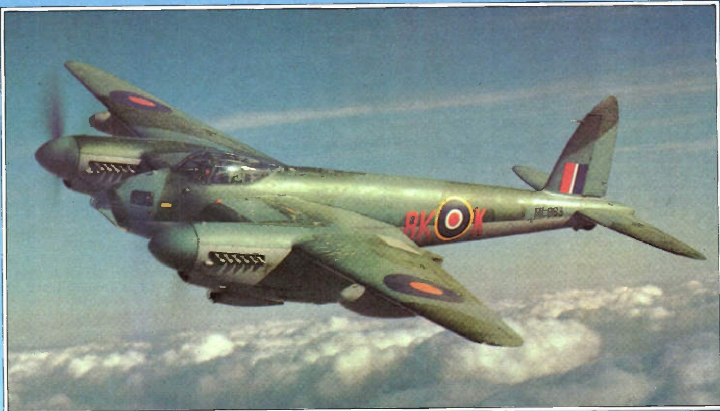
The Mosquito was originally designed as an unarmed bomber which would depend on its superior performance to avoid enemy fighters. It also proved remarkably versatile in other roles, and was a great success for photographic reconnaissance, night fighter, intruder and anti-shiping strikes. Yet the most extraordinary thing about this well-loved and successful aeroplane was the entirely wooden airframe.
