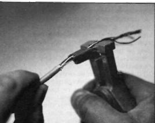
Photo 15. Preparing the four-way screened cable, used to connect the stereo preamp to the front panel controls. Note the use of a Hellerman tool (see text) for the application of expandable sleeving.
