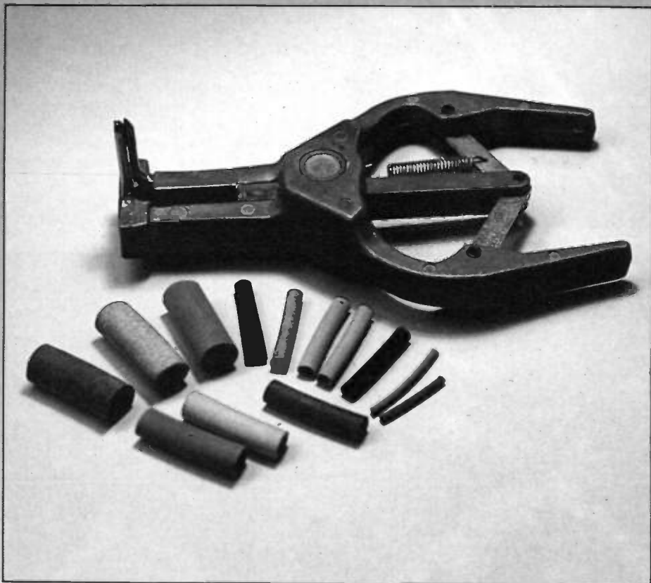
Figure 9. (below) A neat way to finish off cable ends. Photo 14. (left) A Hellerman tool, shown with a selection of expandable rubber sleeves.
