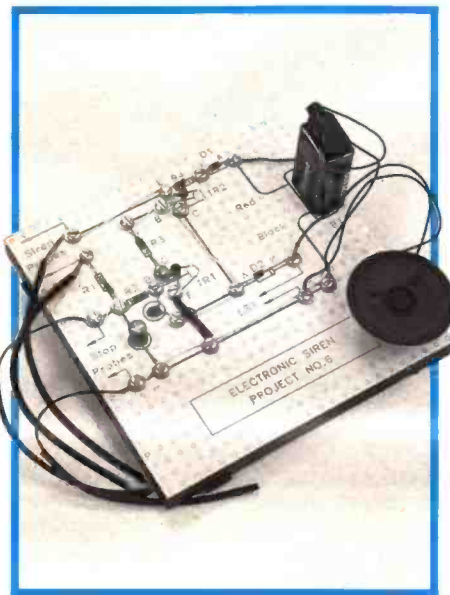
The finished Electronic Siren.
