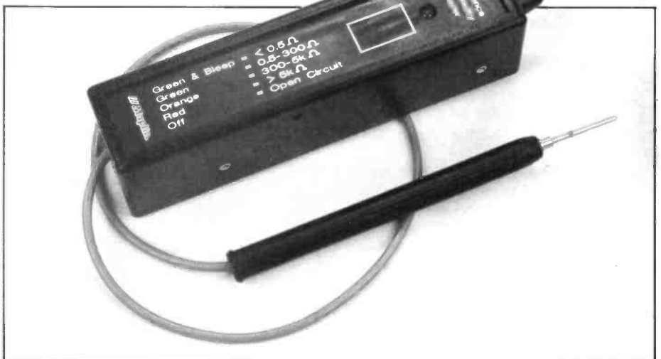
The finished Low-Resistance Continuity Tester.
