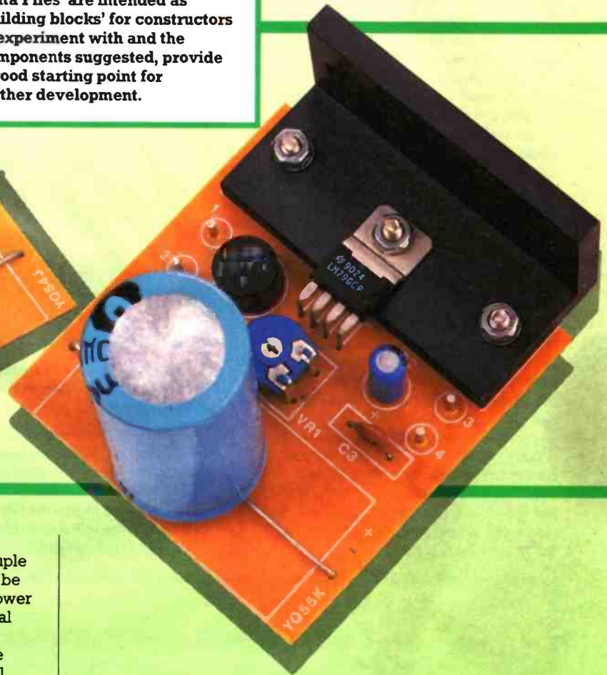
500mA positive (left) and 1A negative (right) variable voltage regulator PCBs.
