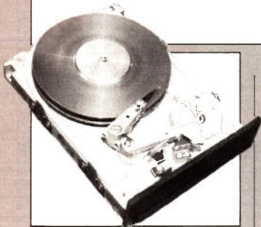
Photo 3. Hard disc drive showing platters and head assembly.
