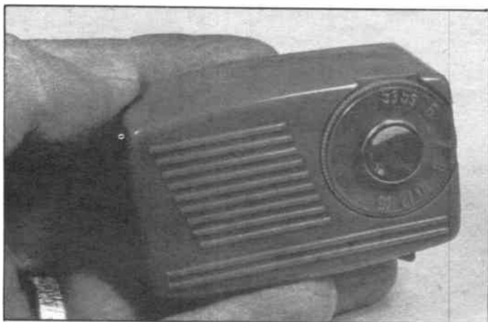
Photo 1. That crystal sets are still made and sold commercially is evidenced by this photograph of the Aiwa AR - 100 'Germanium Radio'. As in the case of traditional receivers of this type, it needs a good aerial and earth and the output drives a high impedance earphone (of the crystal type).
