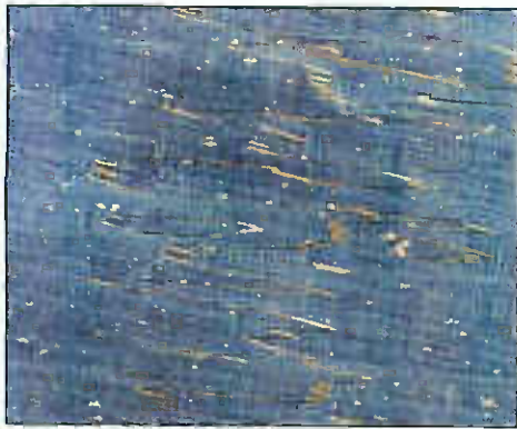
Figure 14. (a) A cell switched one way under an applied electric field. (b) The previous cell switched with the opposite polarity electric field.
