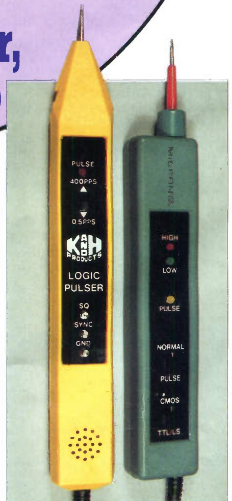
Left: A logic pulser. Right: A logic probe.
