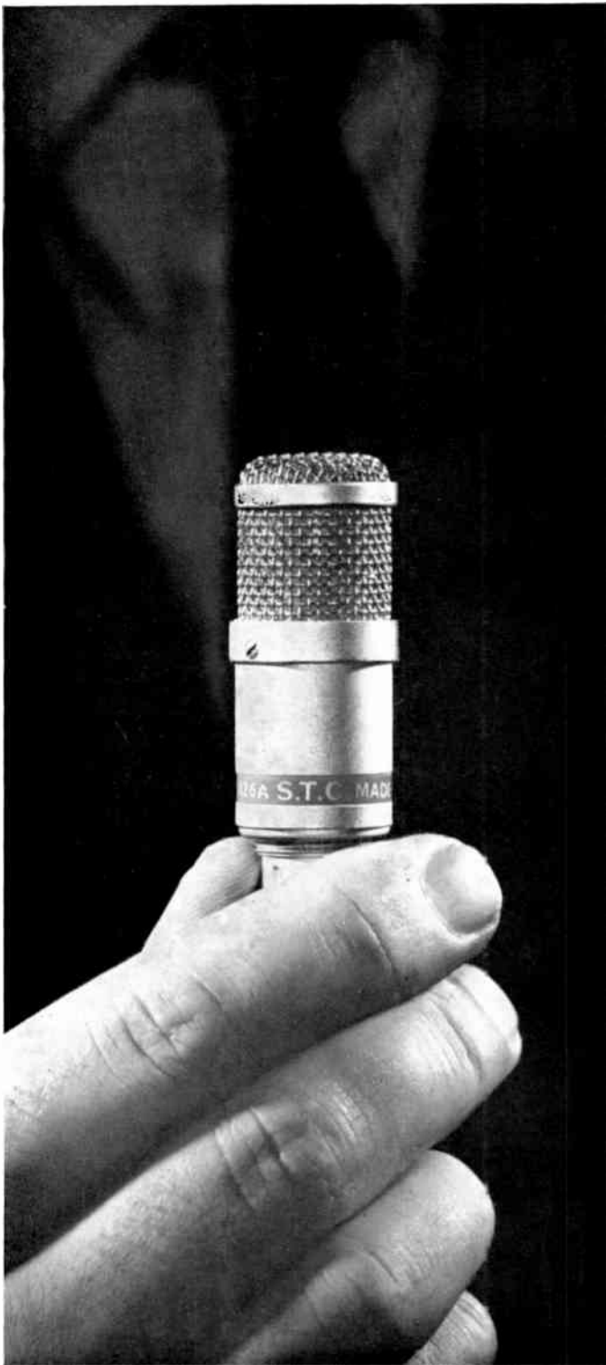
The STC 4126 miniature capacitor microphone
