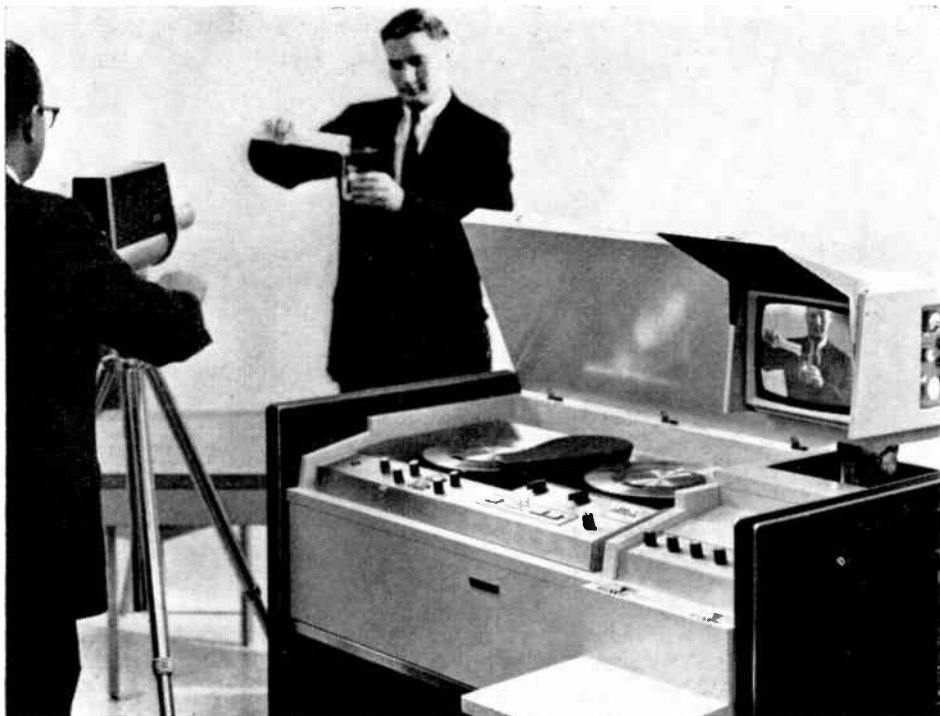
Receiver on Ampex Videotrainer captures sharp image of model conducting classroom experiment. The mobile Videotrainer, which contains a videotape recorder, television camera, receiver and all other equipment necessary for closed circuit television production, is ideally suited for use in education, medicine and the military services. Programmes produced with the Videotrainer may be played back on any number of conventional television receivers for classroom or other remote viewing.
