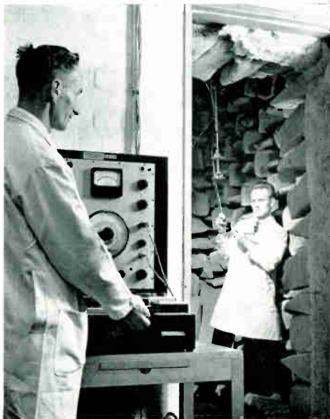
Testing an STC microphone in an anechoic chamber — see story on page 740
