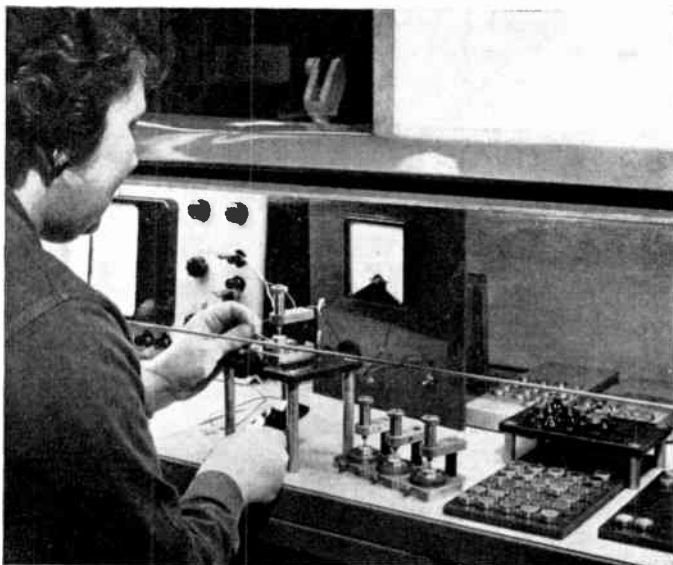
▲ Testing diaphragm tension on capacitor microphone capsule Type 4126
