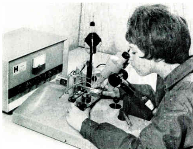
Fig. 7. This manually-operated ultrasonic chip mouter, capable of mounting 250-350 chips per hour. The chips are placed on a mirror plate, orientated, and then picked up by the vacuum tip of an ultrasonic transducer. The substrate is positioned under the transducer, and the chip is then placed on the circuit and bonded into position
