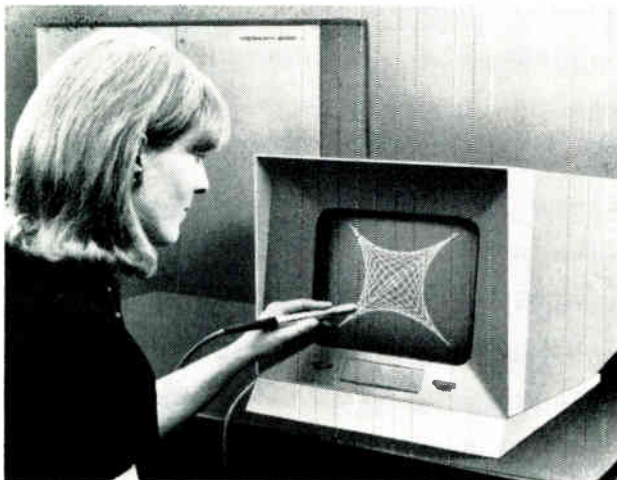
Fig. 3. The table version of the Series-20 display. Using a light pen, information can be fed directly from the c.r.t. face into a computer, where it can be stored, processed or used for on-line applications. Alpha-numeric information on the tube can also be handled in this manner for process control
