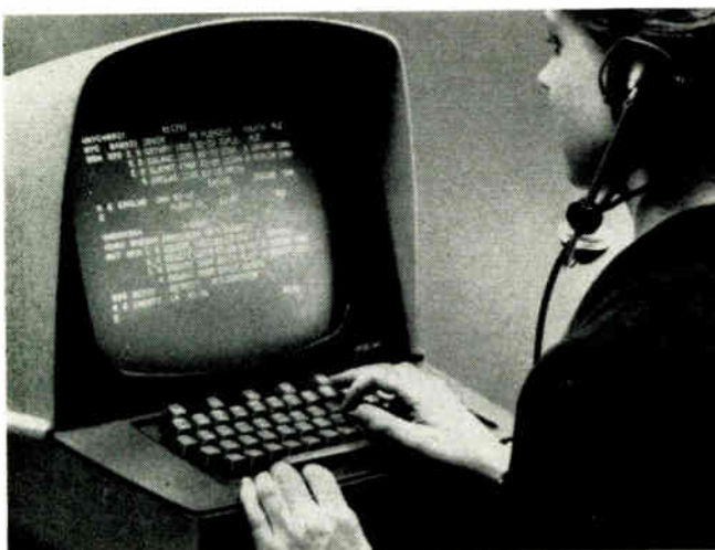
Control Data's remote input/output device (the 6090), a multi-station data-entry and retrieval unit combining an electronic typewriter and c.r.t. display
