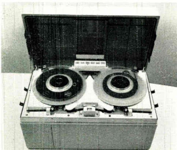
Fig. 2. The ATM-13 digital-tape transport, which produces tape suitable for direct inputting to several computer processing systems
