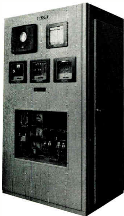
Fig. 6. An on-stream automatic titrator, which contains an analyser (comprising titration vessel, sample and reagent burettes), titration sequence-control units, pH-point indicator and output recorder, all mounted together at the sample point
