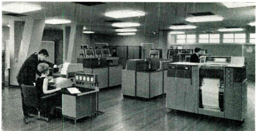
A view of an I.C.T. 1905 computer configuration, for scientific applications. The central processor offers multi-programming facilities and can handle up to four main programmes (each with two sub-programmes) at the same time
