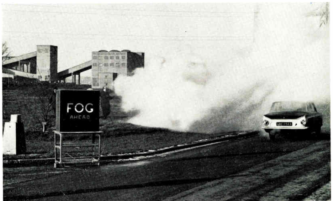
Smoke generators were used to simulate fog for a demonstration of the warning system
