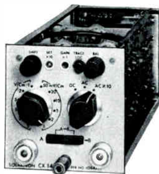
* CX 1442 1 mV/cm DC differential amplifier with a common mode rejection of 60dB. For use with transducers and servo systems etc. An AC \times 10 position gives a sensitivity of 100 \mu V/cm for low level noise investigation.
