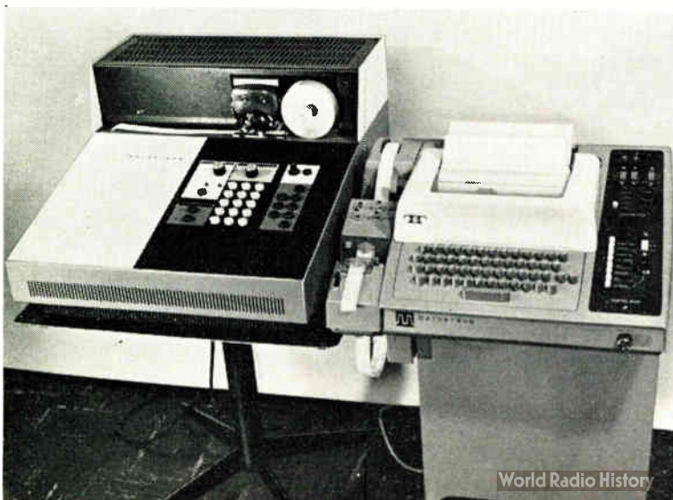
One of the most recent of the many small-sized computers now on the market is the Mathatron, manufactured by Mathatronics and marketed by Calcul S.A. This combines the advantages of automatically-programmed digital computers with those of desk calculators. A number of mathematical formulae, sequences and constants can be pre-wired into the machine and others can be inserted into the ferrite-core programme memory. Accurate results to 8 significant figures are presented on a printed tape. Other output modes are printed pages, punched tape or direct connection via the interface to other equipment. Input is via the keyboard, punched tape or the interface. A number of accessories are available, including the paper tape punch and reader and page printer shown on the right (64)
