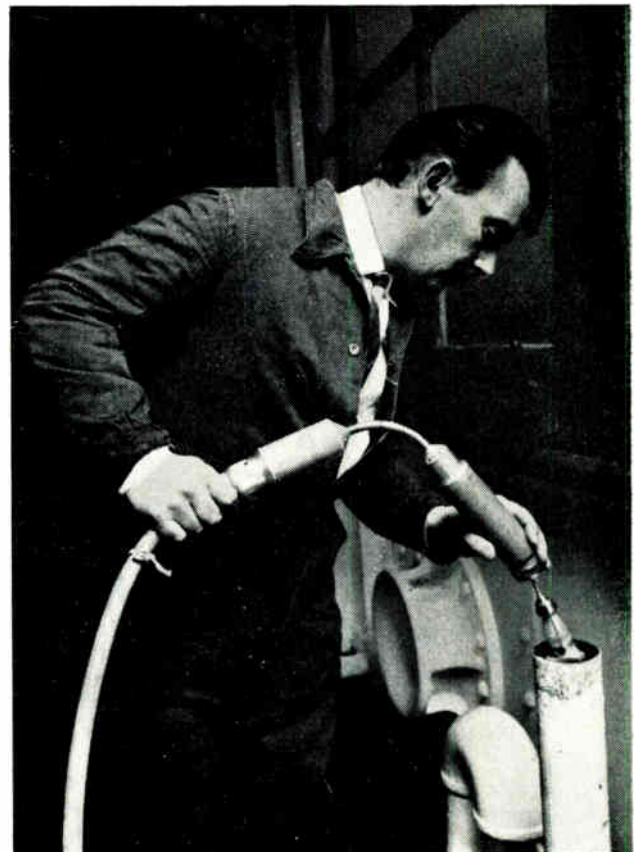
This shows an articulated television camera being lowered down the ventilation pipe of a double-bottomed tank on board the liner the 'Reina del Mar' at Southampton
