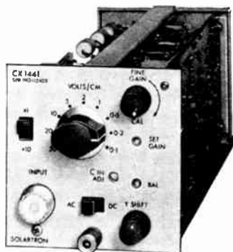
* CX 1441 DC – 15 Mc/s approximately, 100mV/cm, general purpose amplifier suitable for pulse work. Additional \times 10 provides 10mV/cm from DC – 750 Kc/s.
