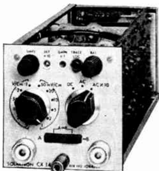
* CX 1442 1 mV/cm DC differential amplifier with a common mode rejection of 60dB. For use with transducers and servo systems etc. An AC \times 10 position gives a sensitivity of 100 \mu V/cm for low level noise investigation.
