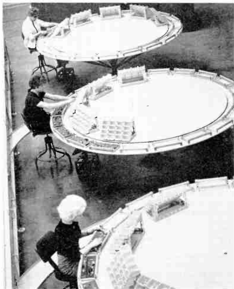
▲ These giant turntables are novel in that they bring mass production efficiency to small quantity runs. The outer concentric rim revolves independently of the inner turntable. Up to twenty circuit boards can be mounted on the outer rim and nests of trays containing components are fixed to the inner turntable. In this way, the operator can first assemble one type of component on to each of the circuit boards and follow with a second type of component and so on. The advantage came from the fact that while the operator will be slow when assembling a component on to the first two or three boards her speed and efficiency are quickly increased
