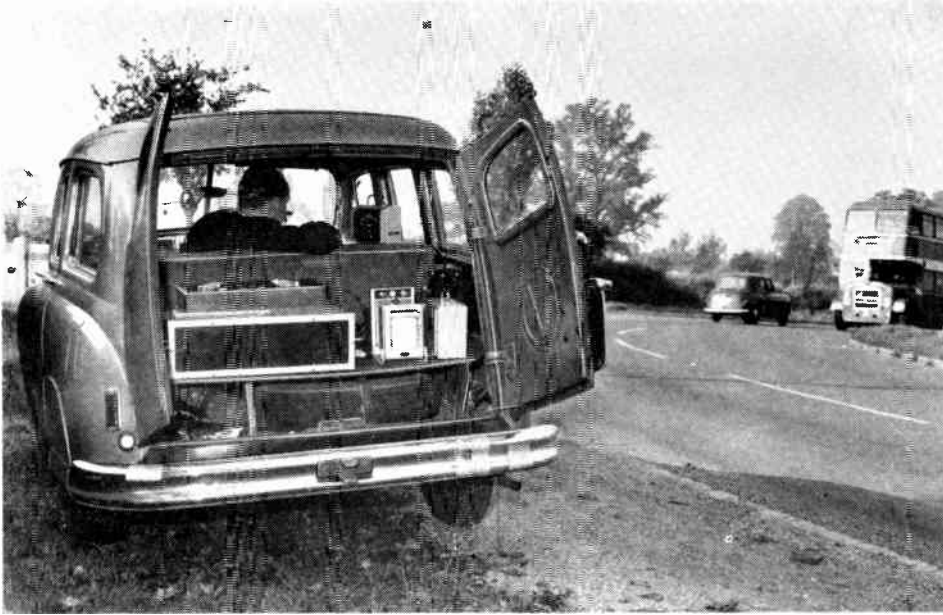
Speed-measuring equipment fitted in the rear of an estate car
