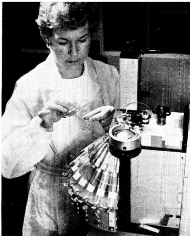
SORTING GERMANIUM WAFERS —Small germanium wafers are sorted at the rate of 3,000 an hour into ten thickness grades by this machine in the transistor division of Standard Telephones & Cables at Footscray, Kent. The machine can detect a difference in thickness of 0.0001 in.
