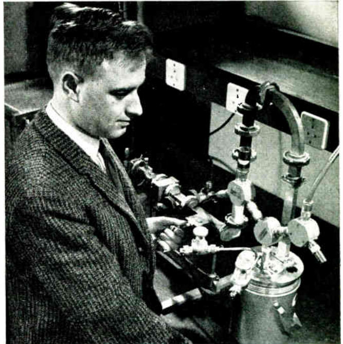
Measuring the gain of an S-band low-noise parametric amplifier. The amplifier is cooled with liquid nitrogen to reduce its contribution to the system noise temperature by a factor of approximately three
