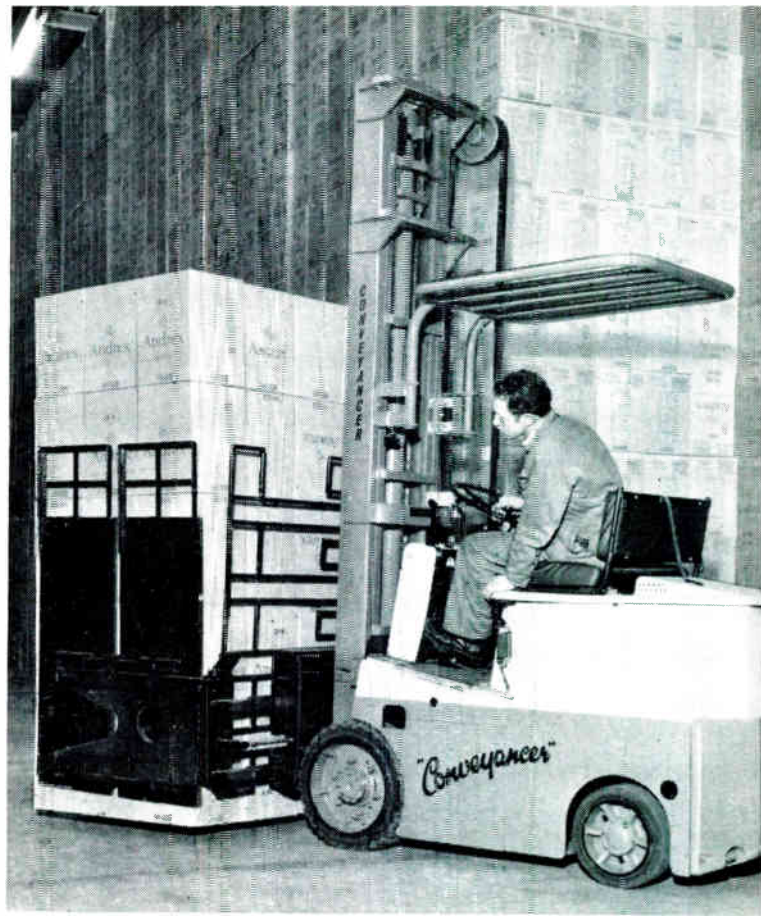
Conveyancer fork truck fitted with thyristor control
