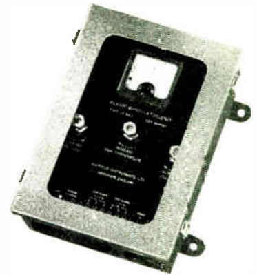
This industrial alarm and indicator unit, type LE463, is one of the devices to be featured by Hatfield Instruments. In conjunction with a sensor, it can be arranged to close relay contacts in the event of either high or low temperature, or both, occurring in the locality of the sensor. The high and low temperature limits can both be pre-set (64)
