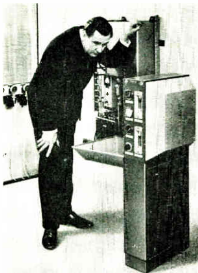
For on-line composition control with laboratory accuracy, Foxboro are showing this industrial chromatograph. Two types of programming units are available for single and multi-stream applications (61)
