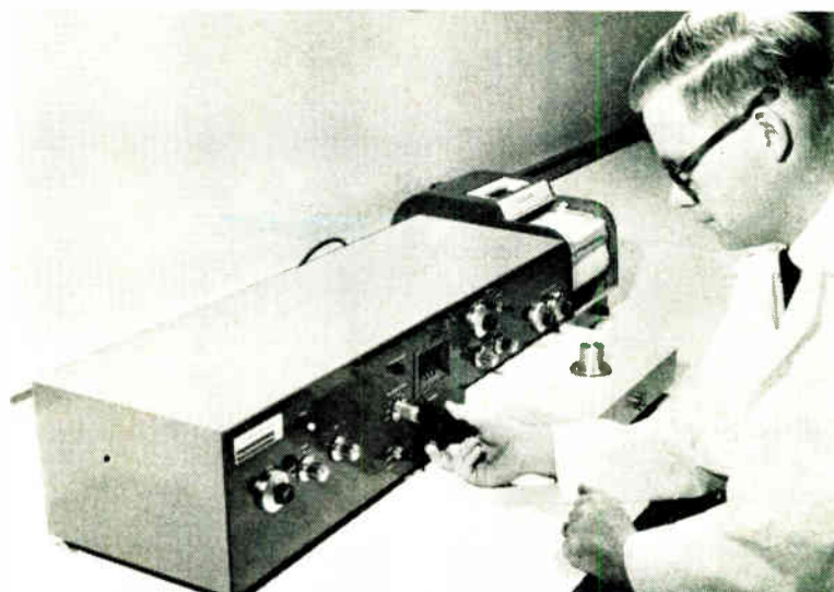
The differential scanning calorimeter in operation
