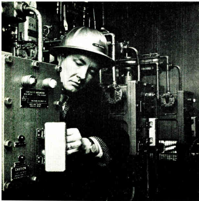
Continuous viscometers manufactured by Elliott-Automation monitor lubricating oil product streams on a clay treatment plant at Esso's Fawley refinery
