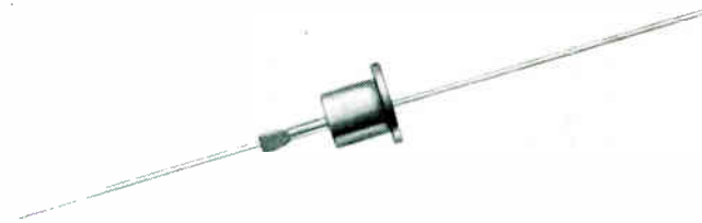
Z3 SERIES ZENER DIODE (actual size)
