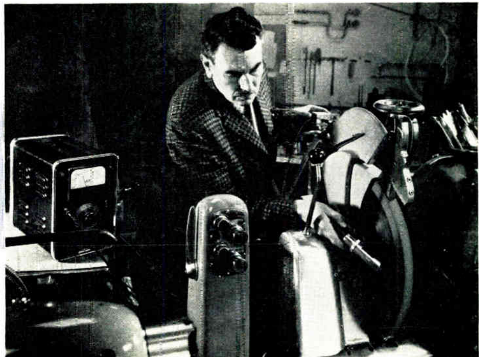
Portable balancing equipment being used to ascertain unbalance on the grinding wheel in situ. (Photo by courtesy of Prince (Kingston) Engineers Ltd.)
