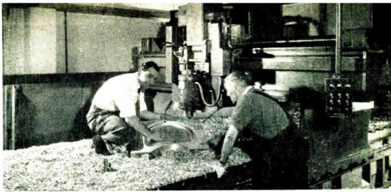
Ceramic continuous profiling machine. The cross-feed screw has a diameter of 4 in.
