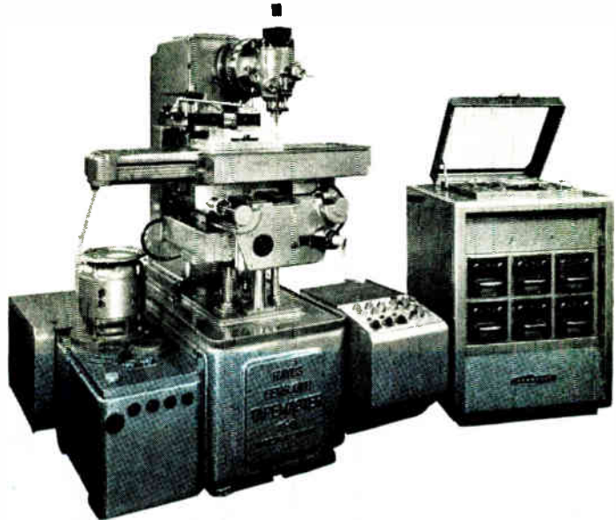
Ceramic continuous profiling machine. The cross-feed screw has a diameter of 4 in.
