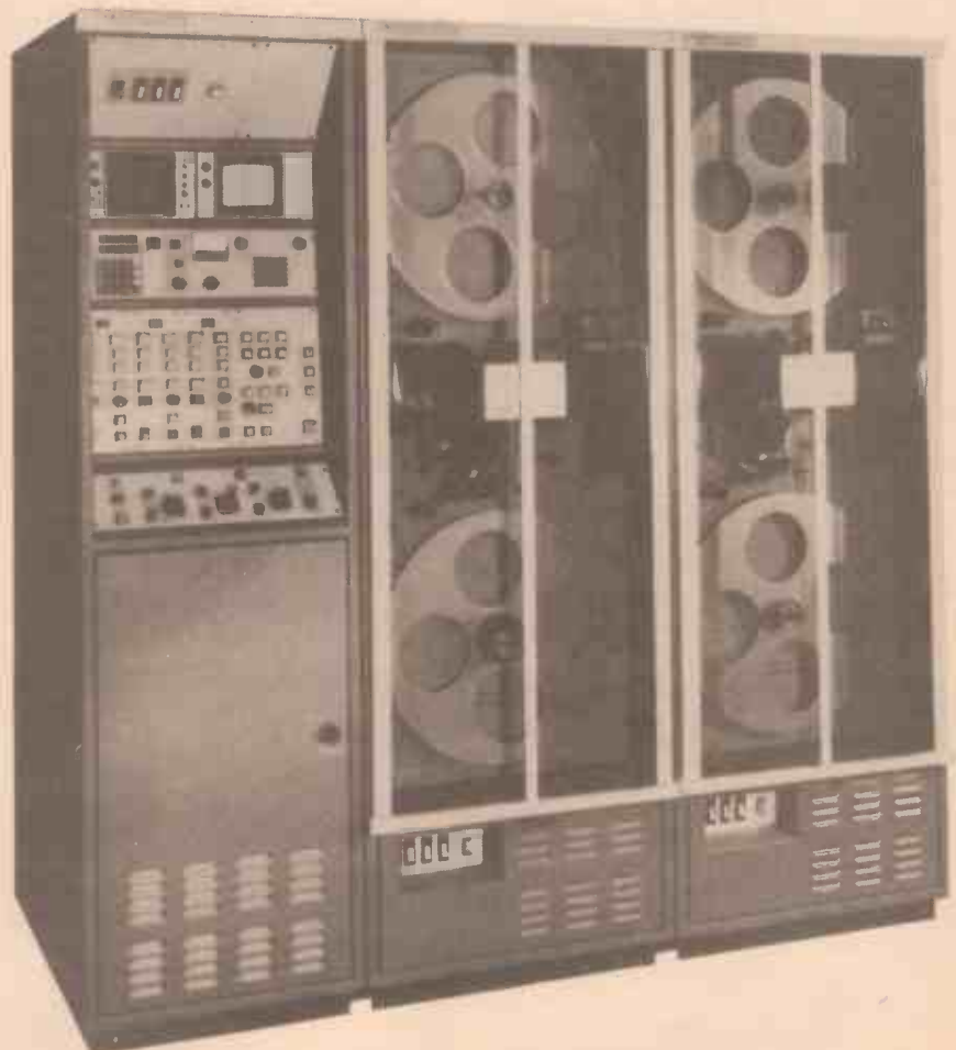
Right: A Rank Cintel ADSI CCD line array machine. Two film transport mechanisms are shown, but the electronics can handle up to three, alleviating the problems of reel changing. The frame store uses 64K RAM chips, and among the features of this advanced machine are a dirt concealment circuit, which uses infrared sensing to locate dirt and scratches, and an automatic colour correction circuit.
