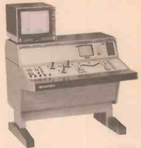
Not Mission Control Houston, but a remote control desk for use with the Rank Cintel Mk III Telecine. Note the colour correction joysticks in prominent view.
