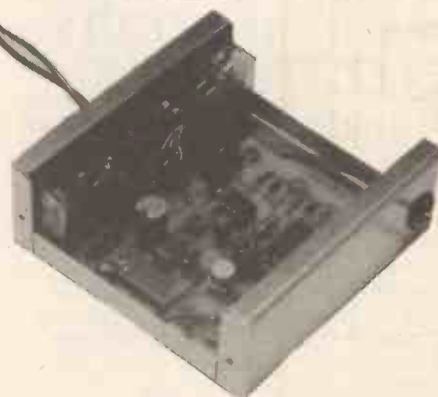
Figure 1. The circuit, using a 555 timer and 4093B Schmitt trigger.
