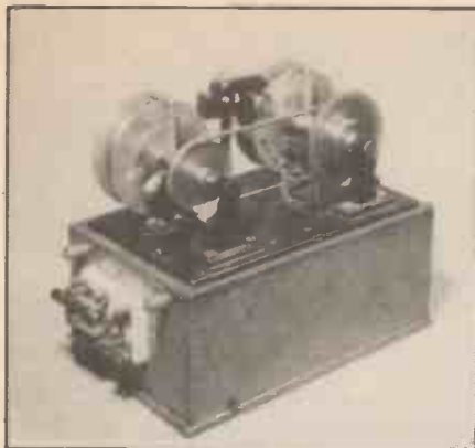
Pulsen's "Telegraphone" was patented in the US in 1898 and used mainly as a dictaphone. "Hifi" had yet to be invented!
