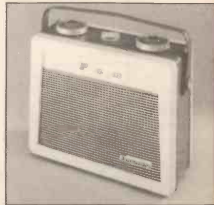
A PAM transistor radio dating from 1956. As today, the physical size was determined by the need for a relatively large loudspeaker.
