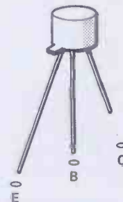
Figure 5. Transistors can be fitted more easily, and errors reduced, by cutting the wires to unequal lengths. The emitter wire is left full length, the base is cut shorter and the collector the shortest. They are inserted in the same order.
