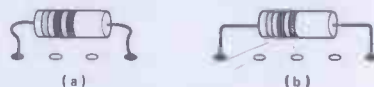
Figure 3. When a component straddles several holes on a matrix board count the number as it is fitted. It is not so easy to check when the part is in place.
