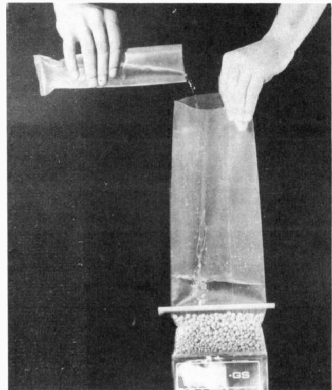
2). Remove the top clip and add 250 ml of warm water. If you have not got a measuring jug, use the polythene bag supplied. It will hold 250 ml when full to within an inch of the top.
