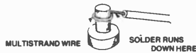
Fig. 25. 'Wicking' is caused by solder running back up multistrand hookup wire. This makes the wire brittle at the joint and movement may break it.
