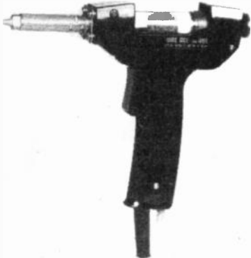
Fig. 40. This Hako 'Vac Ace' desoldering tool from G.E.S. employs a small vacuum pump to draw molten solder from the joint into the glass barrel atop the gun handle. A steel wool wad absorbs the solder. This tool is particularly effective on through-hole plated PCBs.
