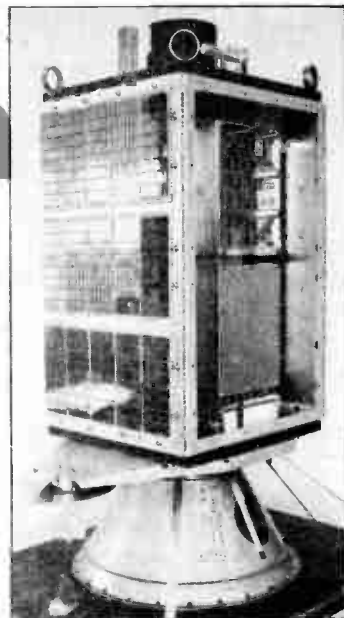
View of UOSAT's structure. One of the solar cell panels has been removed to show four of the sixteen boxes machined from solid aluminium. Each box contains two printed circuit boards: about 400 PCBs are used in the spacecraft
