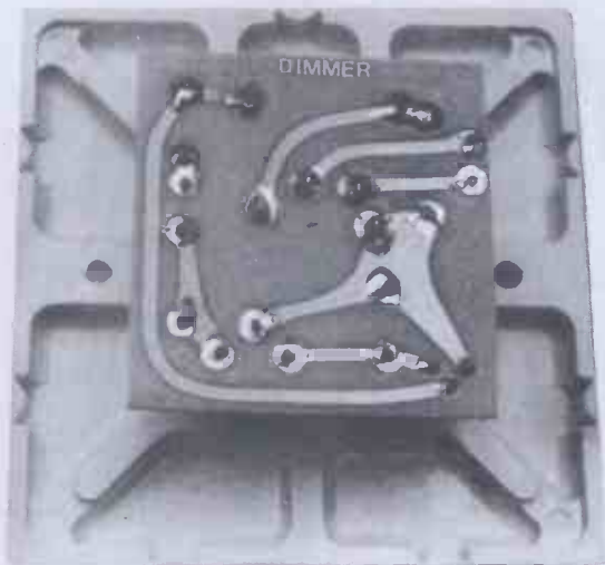
A view of the completed PCB mounted on the MK blanking plate. This gives you some idea how small it is.
