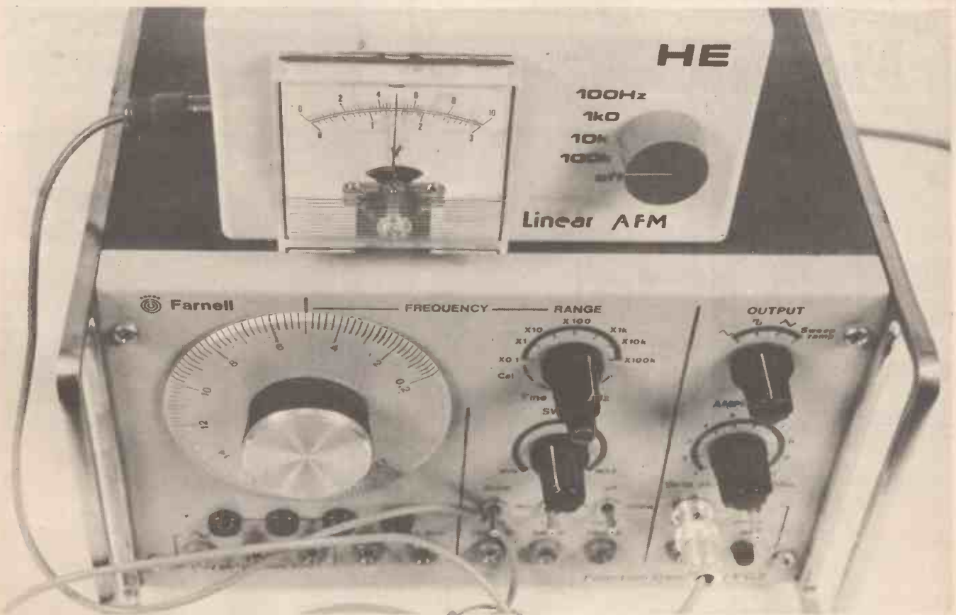
Calibrating the HE Audio Analogue Frequency Meter against the workshop signal generator. For those without any test equipment an alternative method is outlined in the text
