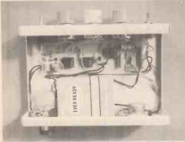
A bird's eye view of the Siren showing the component layout. Note the phono output socket on the rear panel.
