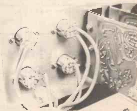
Close-up of the connections to the input sockets, note the use of screened lead
