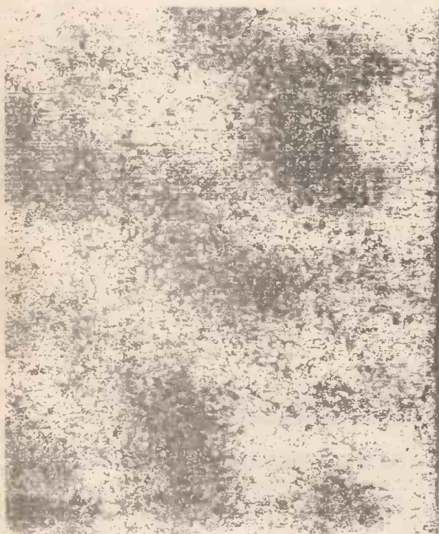
Heating pattern in a microwave oven (recorded in a horizontal plane 4in. above the cavity bottom). Dark areas indicate strong heating, light areas weak or no heating. (Courtesy Western Dynamics Ltd.)
