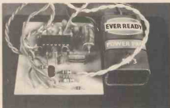
Close-up of the PCB and battery, the PCB is mounted on to the case by double-sided sticky pads.
