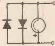
Fig. 13. A moving coil meter can be given a limited degree of overload protection by connecting two germanium diodes as shown.
