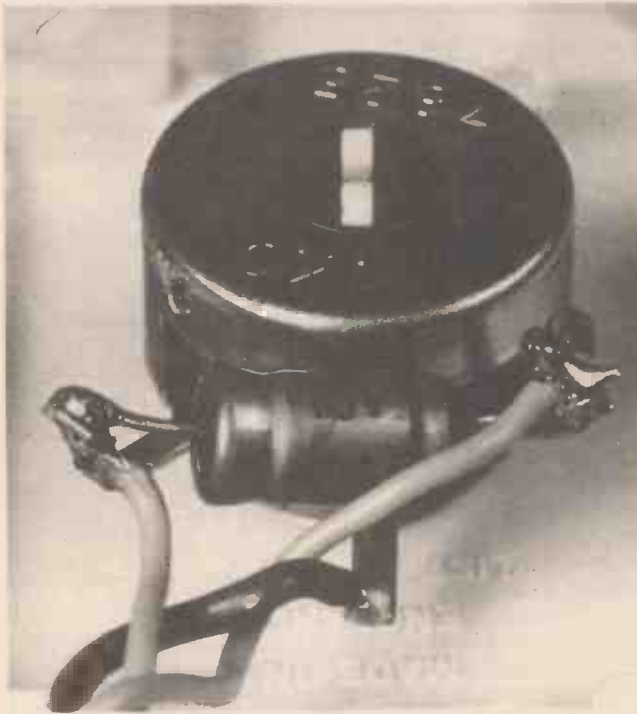
Mounting capacitor C1 on the control potentiometer RV1.
