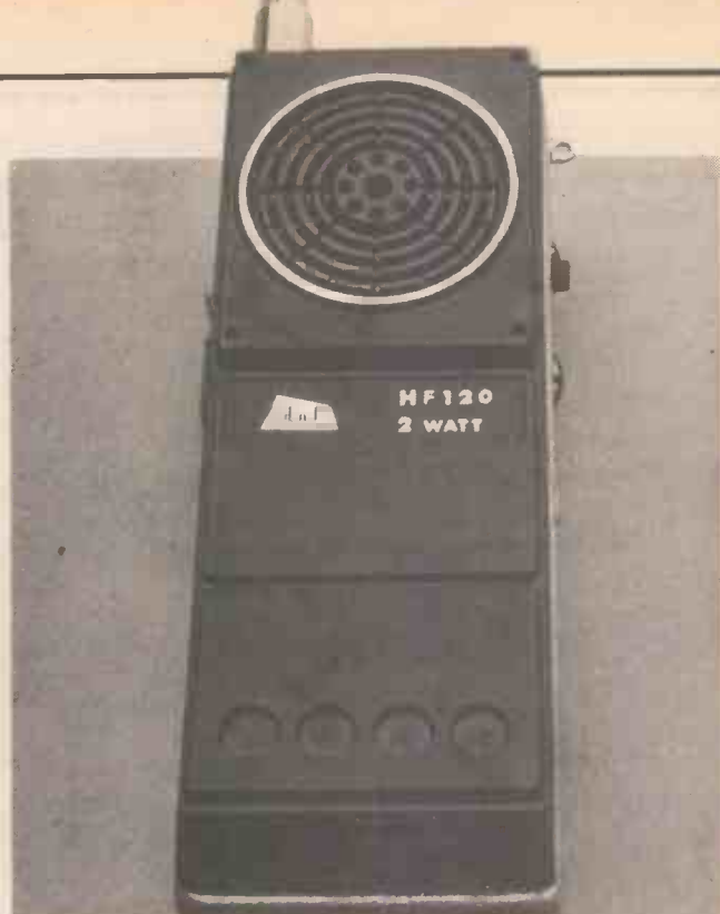
A Walkie-Talkie radio working at CB frequencies, these handsets are usually only capable of operating at very limited power, the one shown is an exception using 2 watts RF power.
