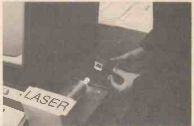
Maplin Electronics had on display a small laser. This was set up as a sort of fairground novelty — the idea being that you had to move the cut-out along the beam to the end without cutting the beam. A small electronic counter with a photo-electric input measured the time the beam was interrupted for. The laser was perfectly safe and wouldn't burn a hole in anything — well, that would spoil the purpose of the game!
