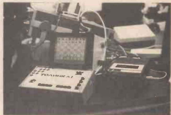
Another Electronics Today project, the Tcholinka chess recorder. This machine was used by the BBC in their coverage of the Korchnoi/Karpov chess match. The name comes from the Russian — Korchnoi named it (he also uses one). The machine is capable of storing an entire game in its memory and can record it onto a cassette tape for future reference. It also allows the game to be played from cassette with a commentary — thus allowing a professional player to review all the common openings, for instance, the day before a game.
