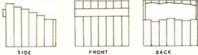
SLEEPER BUILT BUFFER STOP
