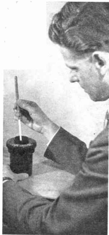
Testing temperature of the solution to ensure strict application of the correct developing time
