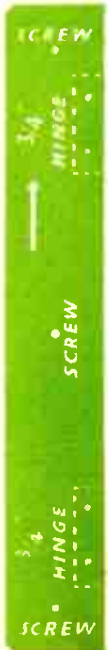
BACK RAIL TO TAKE STRUT. CUT ONE 3/8 in. AND GLUE BEHIND BACKING PIECE TO GLASS.
