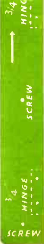
BACK RAIL TO TAKE STRUT. CUT ONE 3 3/4 in. AND GLUE BEHIND BACKING PIECE TO GLASS.
