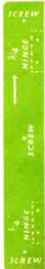
BACK RAIL TO TAKE STRUT. CUT ONE 2 1/2". AND GLUE BEHIND BACKING PIECE TO GLASS.
