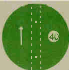
BOILER, END DISC. CUT TWO 3/16in.
