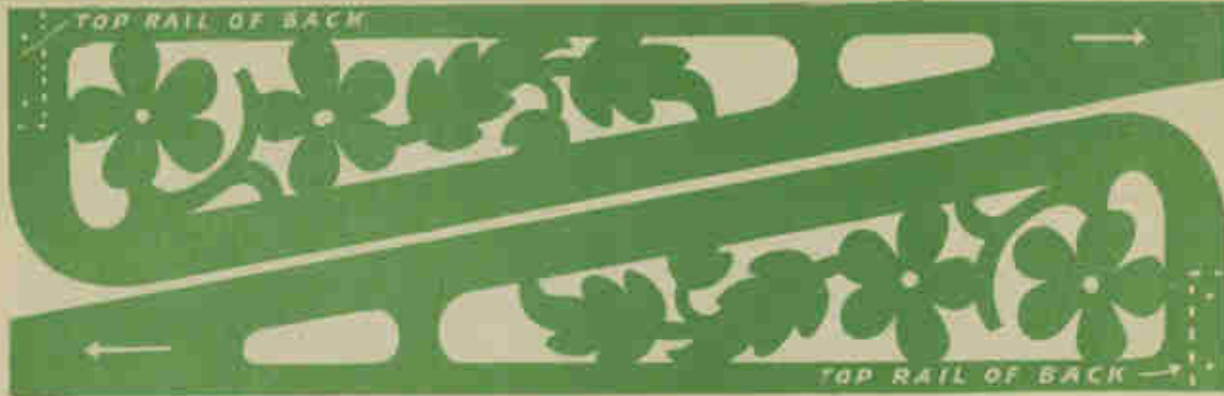
SIDE RAILS OF LID. CUT THE TWO FROM 3/16IN.
