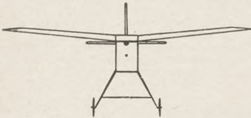
High-wing model, with (large dot) centre of resistance, and (small dot) centre of fuselage
