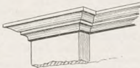
How the moulding is fitted round the projecting pieces
