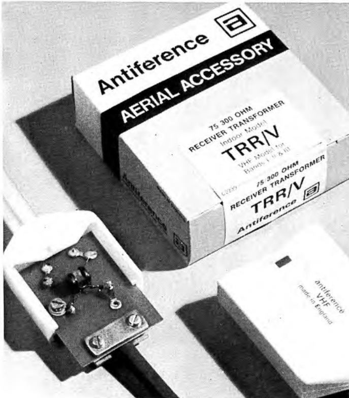
Fig 5 75/300 ohm receiver transformer to match 75 ohm coaxial downlead into a 240/300 ohm twin 'balanced' input. Courtesy: Antiference Ltd.
