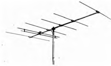
Fig. 6 A six-element array required for fringe area reception.
