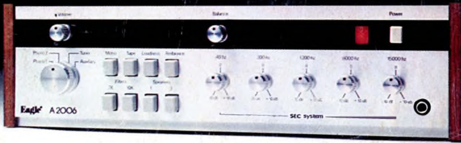
A 2006 - (Sound effect control system) Output power: 20 watts RMS per channel into 8 ohms. Frequency Response: 15Hz-36KHz \pm 2dB. £85.00 Ex. VAT.
