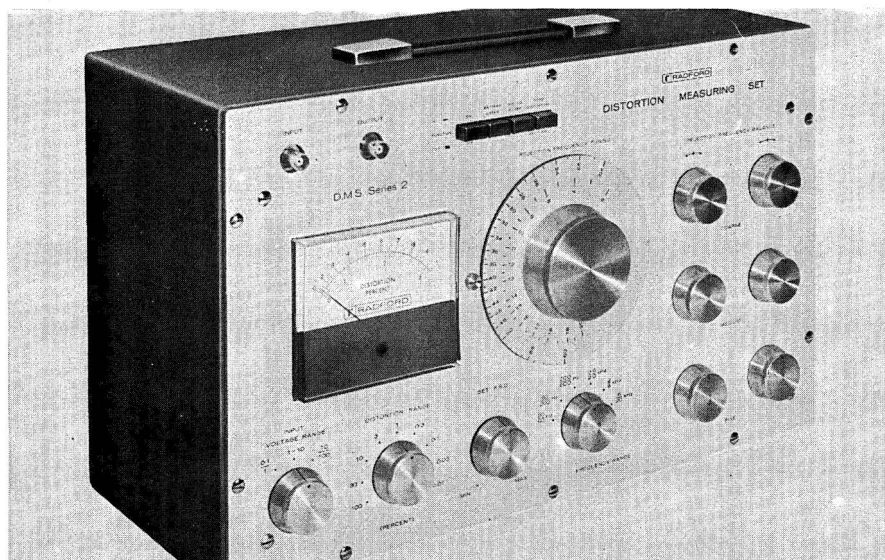
Distortion measuring equipment type DMS from Radford Audio
