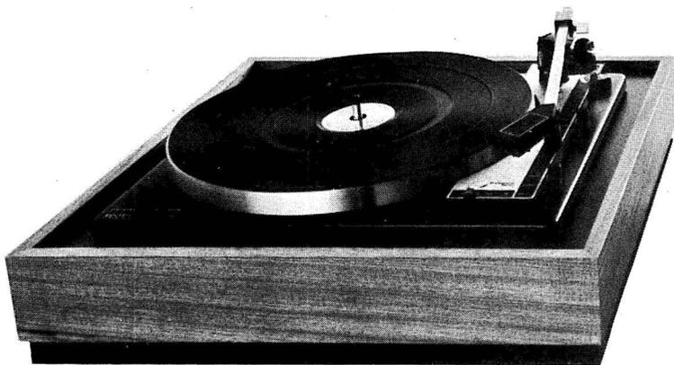
The HT 70 is a luxury single player with a fully counterbalanced pickup arm, deep rim 4½ lb die cast turntable, rotating record stub spindle, viscous damped cueing device, slide-in cartridge holder, anti-skate control, and a 4 pole dynamically balanced synchronous motor.
