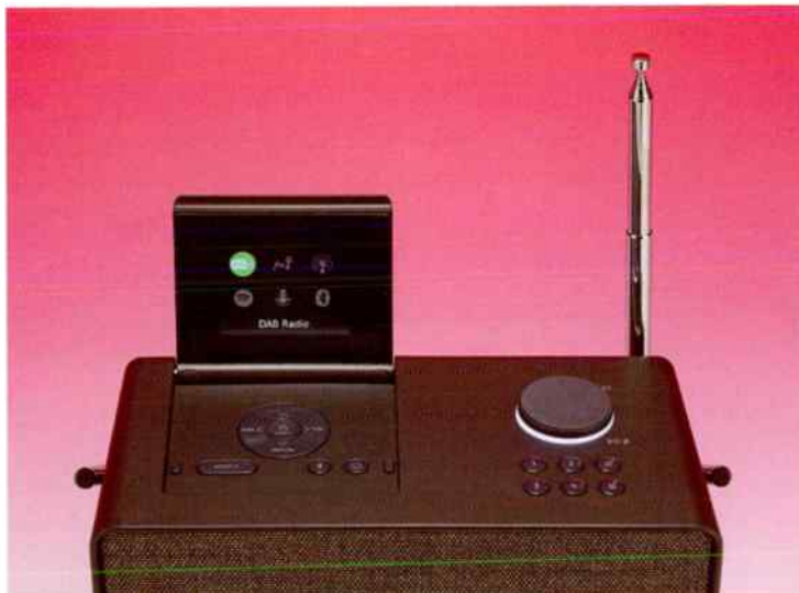
The flip up screen reveals buttons to access the various menus, such as the source select menu shown here. It folds away to preserve the elegant look of the system.
