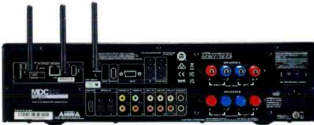
At left two MDC2 card slots, one with BluOS-D card equipped wi-fi and Bluetooth transmit aerials. Top centre are control ports and, below, analogue and digital inputs, including HDMI with ARC for TV, preamp output and Phono input.
