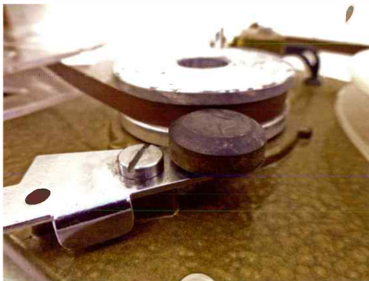
When the record player's turntable is revolving, a lever brings this small rubber pinch roller into contact with the capstan shaft to pull the tape through its unusual path.
