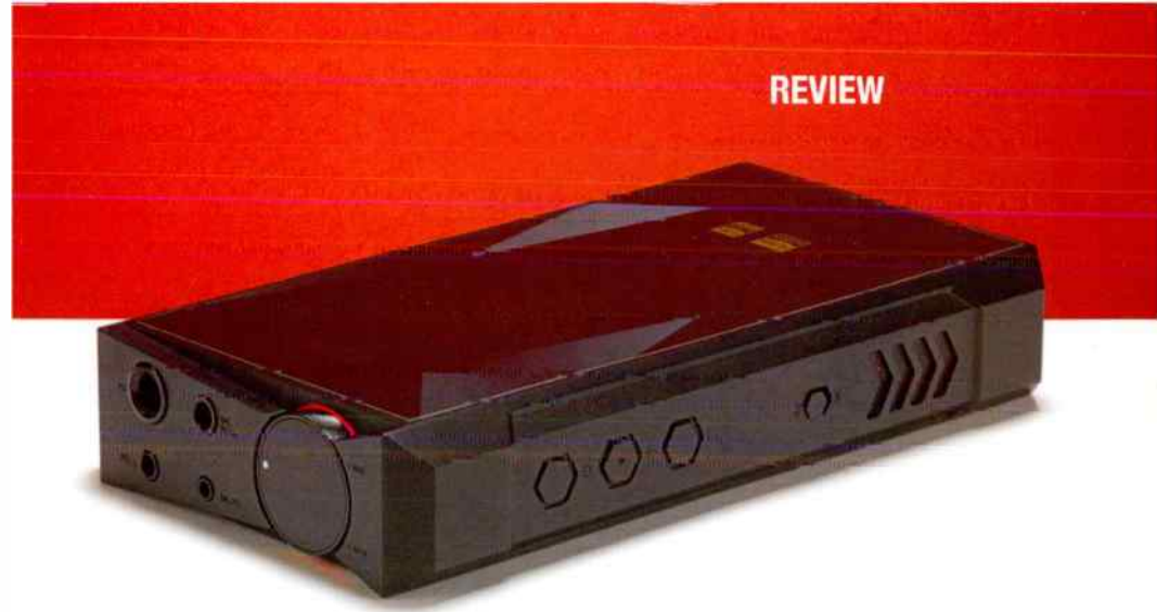
At top a big rotary volume control and four headphone sockets, all different. At side a power button and volume up/down.
