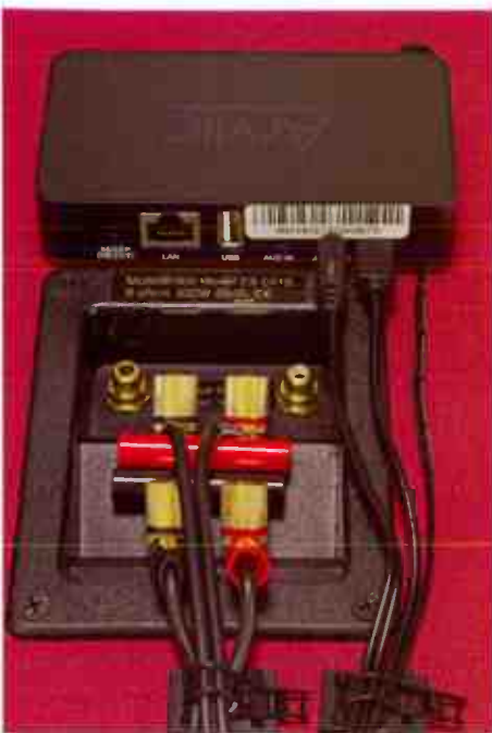
The underside of the Arylic S10 carries a variety of input sockets, including RJ45 for Ethernet and USB for Flash memory storage. At right analogue output and power input, plus Bluetooth aerial cable.
