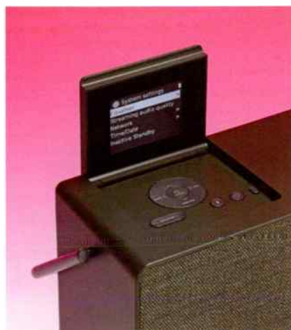
The System settings menu offers various sub-menus. Select the Equaliser menu to adjust treble and bass.
