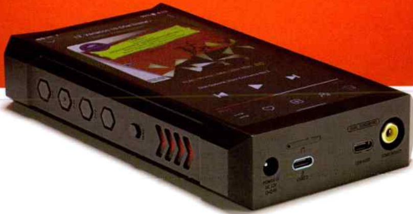
On the base a coaxial 12V d.c. power input (left) a USB C for computer connection and USB C for power, plus S/PDIF in/out.
