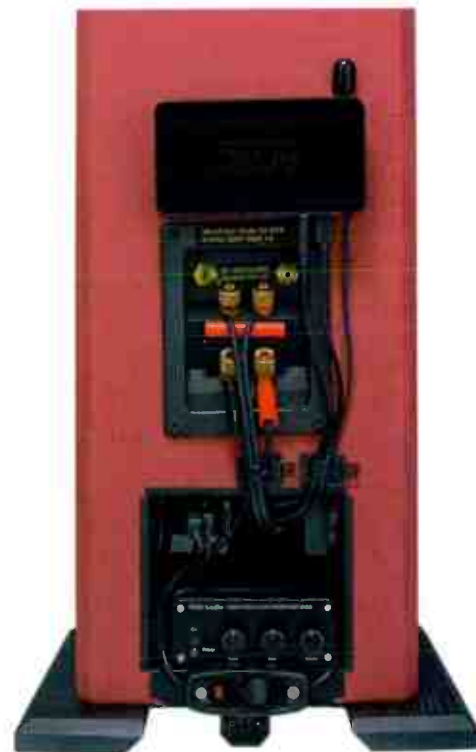
The small Fosi Audio Class D 35W stereo amplifier with uncalibrated bass, treble and volume controls, plus toggle power switch. Below is a main power switch and underneath that a mains power input.
