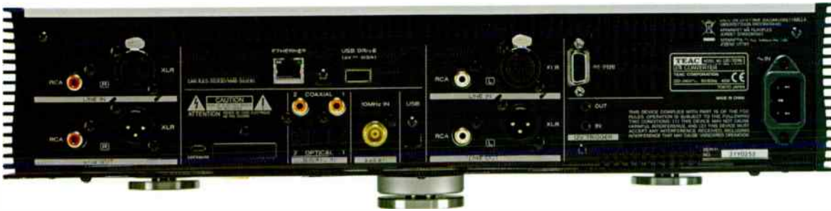
Analogue outputs and inputs at left and centre. Between them and at top, the RJ45 ethernet socket for internet connection with, alongside, a USB mass storage socket to accommodate Flash memory music file storage.
