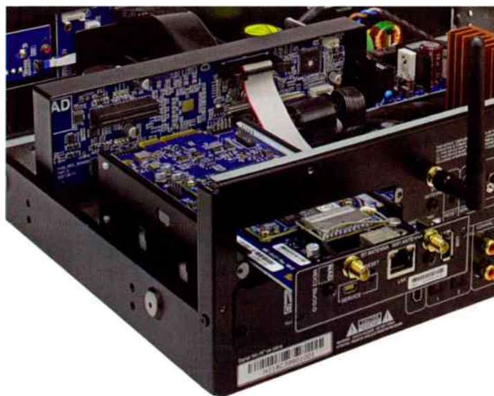
NAD's MDC2 BlueOS-D plug-in board with gold plated sockets for Bluetooth (transmit) and wi-fi aerials, both supplied. The board slides in on white plastic rails and is secured with two screws. Two boards can be accommodated. Easy to fit if care is taken to engage board with side rails.
