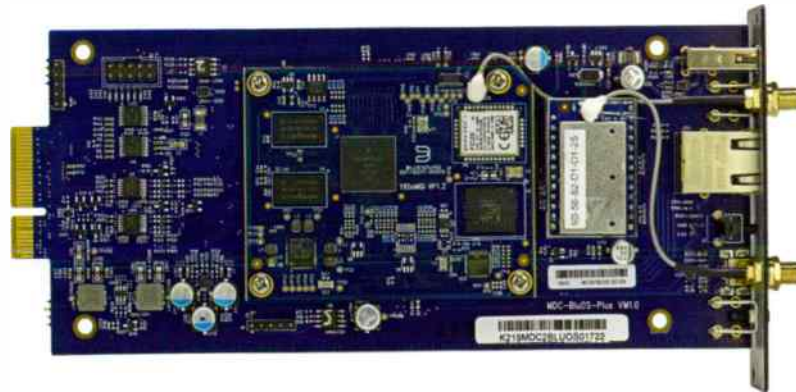
NAD's MDC2 BlueOS-D board that comes as an optional user upgrade. It carries Bluetooth transmit and wi-fi aeriels connected to gold plated sockets at right. At centre an RJ45 ethernet socket and at top a Dirac loudspeaker tuning USB input. The board is massively complex, full of hi-tech chips.
