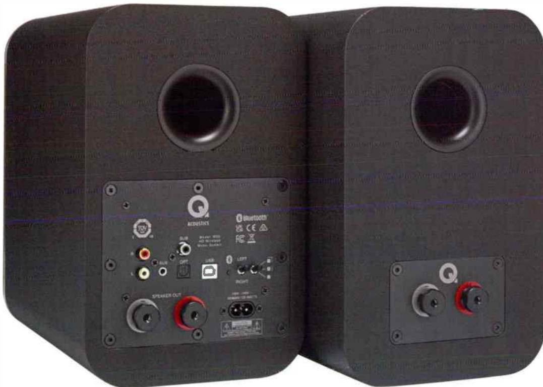
An active loudspeaker (left) carries a stereo power amplifier, with an output through 4mm sockets to the passive partner (right), via a cable terminated with 4mm banana plugs. The active speaker carries a USB B input for computer connection, as well as optical and electrical inputs, plus analogue inputs through RCA phono sockets. At right a three-position toggle switch selects Wall, Corner or Free Field placement, adjusting bass response to suit. The amplifier's electrical response measured flat at Wall.
